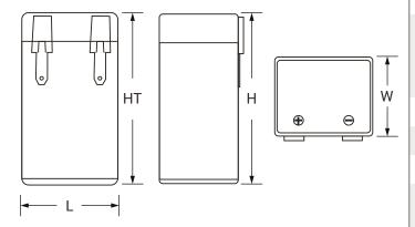
**W**: 1.46 (37) **H**: 2.99 (76) HT: 2.99 (76) Tolerances are +/- 0.04 in. (+/- 1mm) and +/- 0.08 in. (+/- 2mm) for height dimensions. All data subject to change without notice.
