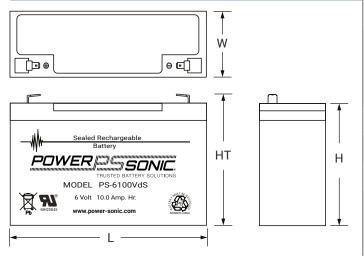
**W**: 2.00 (51) **H:** 3.70 (94) **L:** 5.94 (151) Tolerances are  $\pm$  -0.04 in. ( $\pm$ -1 mm) and  $\pm$ -0.08 in. ( $\pm$ -2 mm) for height dimensions. All data subject to change without notice.
