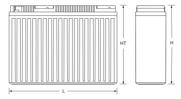
15.50 (394) **W**: 4.33 (110) **H**: 11.20 (285) **HT**: 11.20 (285) Tolerances are +/- 0.04 in. (+/- 1mm) and +/- 0.08 in. (+/- 2mm) for height dimensions. All data subject to change without notice.
